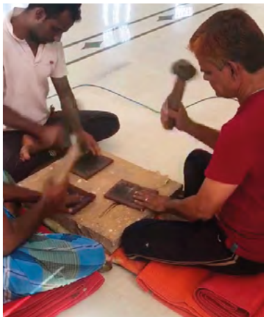
The leather pouches are hammered hard and consistently for a few hours so that thin gold leaves are formed in-between the pages.
