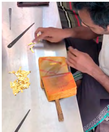
Placing the small gold pieces in-between pages of a booklet. On touching a page it felt like soft and malleable skin that could easily withstand intense manual hammering. For obvious reasons they refused to give me a sample page.
