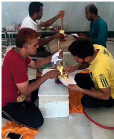
The following day the gold leaves are carefully removed and placed on to a metal base on which mercury could have been applied. The gold varakh is set with the help of a gas fire gun.
